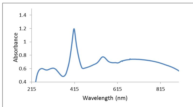
Fig. 2b UV-Visible spectrum of ZnTPyP
