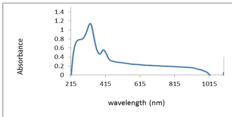
Fig. 2a UV-Visible spectrum of TPyP
